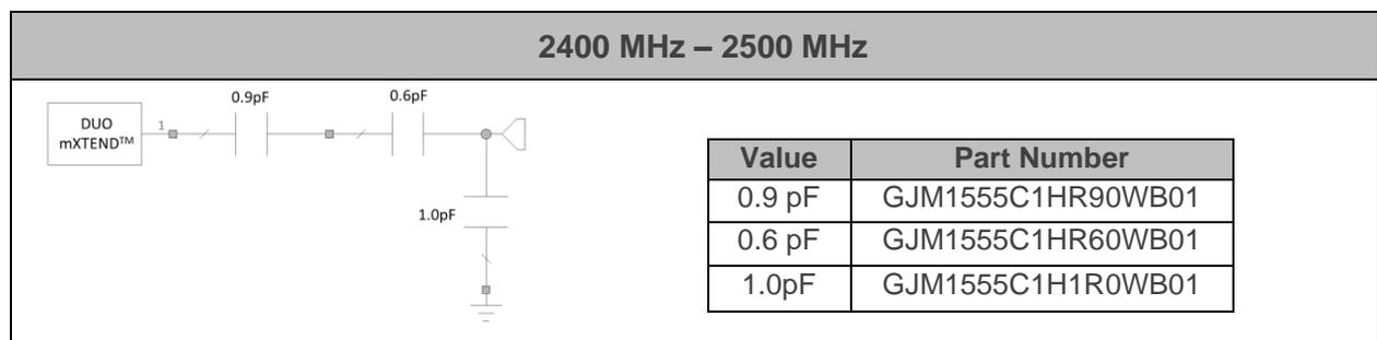
**Figure 2** – Matching Network implemented in the evaluation board (Figure 1).
