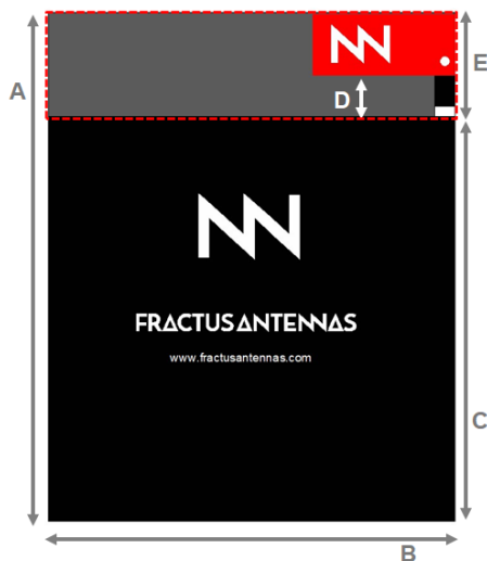
Figure 1 – EB_NN03-320-UWB. Evaluation Board providing operation at UWB (from 3.1 GHz to 10.6 GHz).
