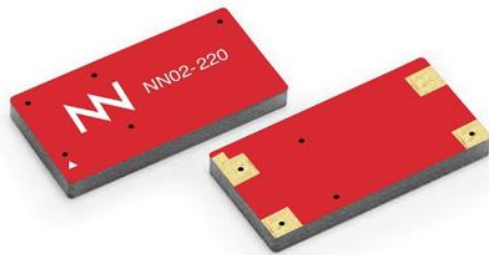
ALL mXTEND™ chip antenna component NN02-220
