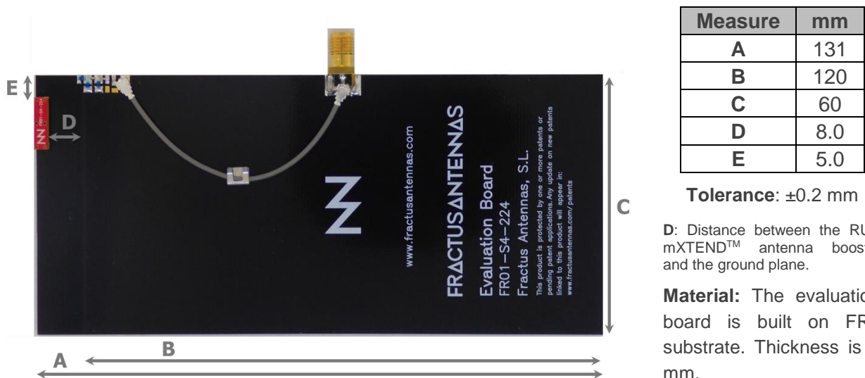
Figure 1 – EB_FR01-S4-224-1B-2R-1P. Evaluation Board providing operation from 824 MHz to 960 MHz and from 1710 MHz to 2170MHz.
