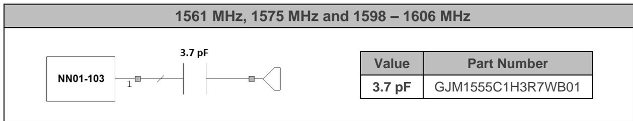
Figure 5 – Matching Network implemented in the Evaluation Board (Figure 4).
