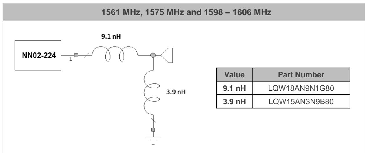
**Figure 2** – Matching Network implemented in the Evaluation Board (Figure 1).
