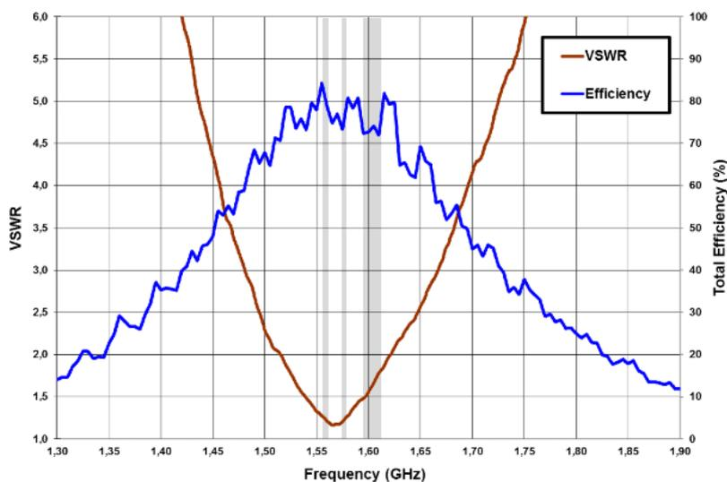
Figure 6 – VSWR and Efficiency vs. Frequency (GHz).
