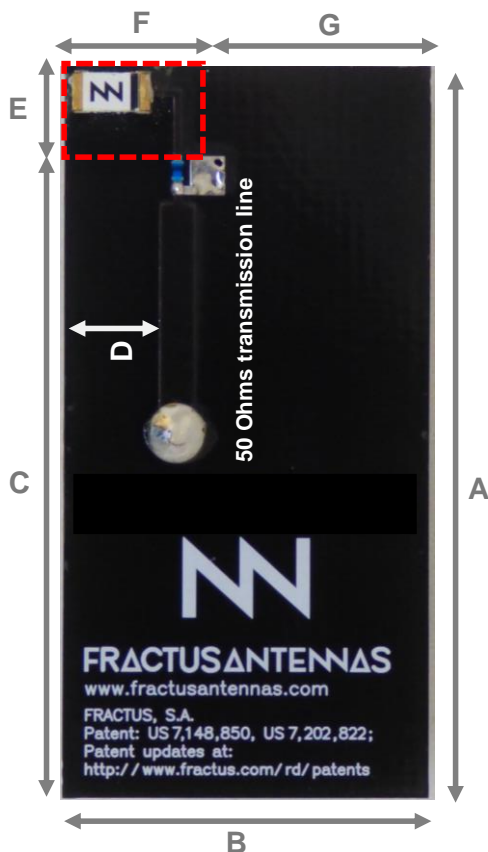
Figure 1 – Example of the Micro Reach Xtend™ antenna in a 120 x 60 mm PCB.
